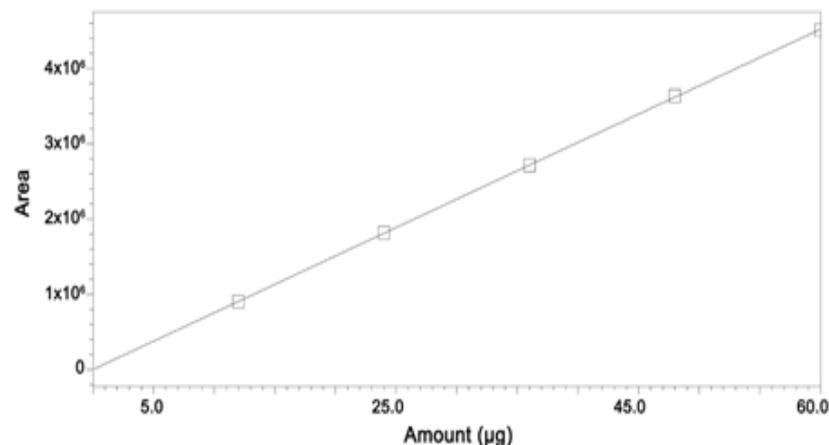
**Fig. 4.** Calibration curve of artemisinin standard (Dilutions of stock solutions of artemisinin standard: 1.0 mg/mL were prepared for further analysis by HPLC and construction of the calibration curve:  $r^2=0.999933$ ).
