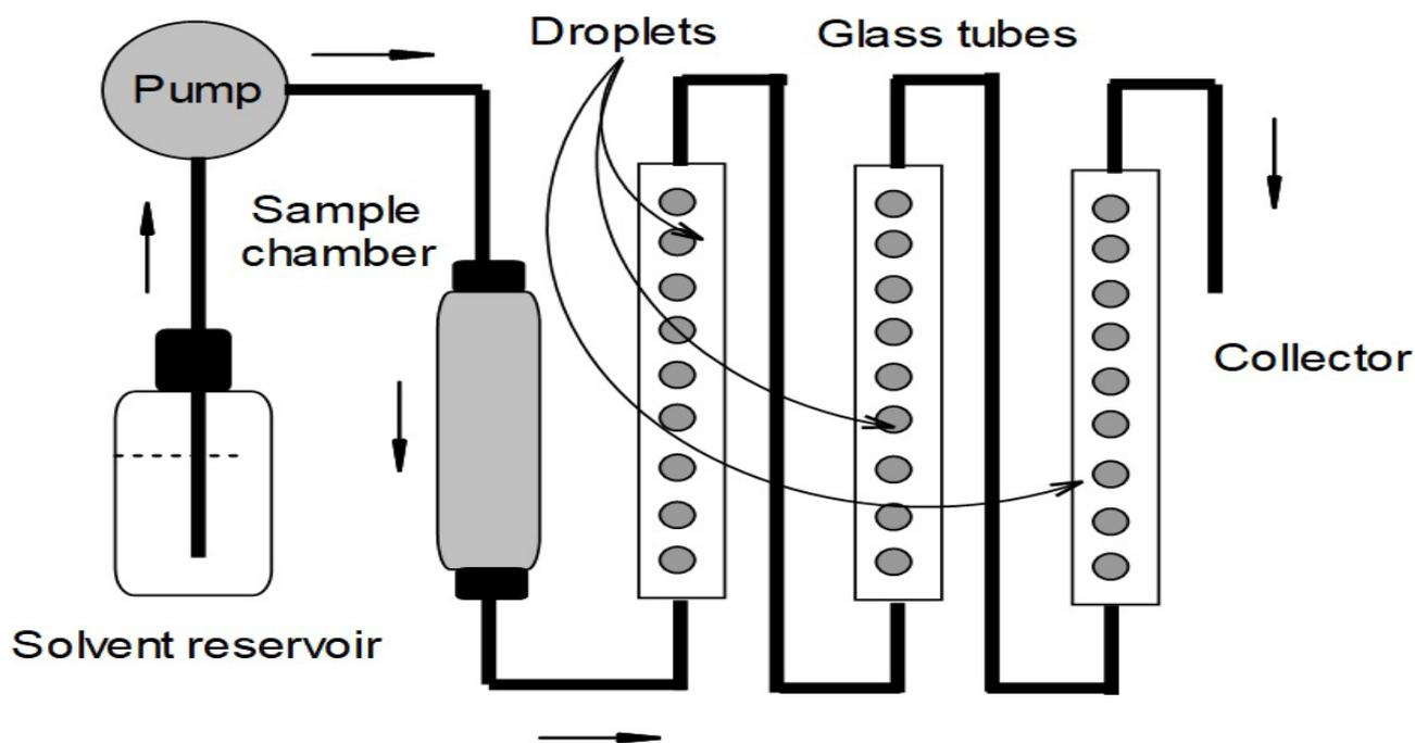
**Fig. 1.** A schematic diagram of droplet counter current chromatographic (DCCC) system.
